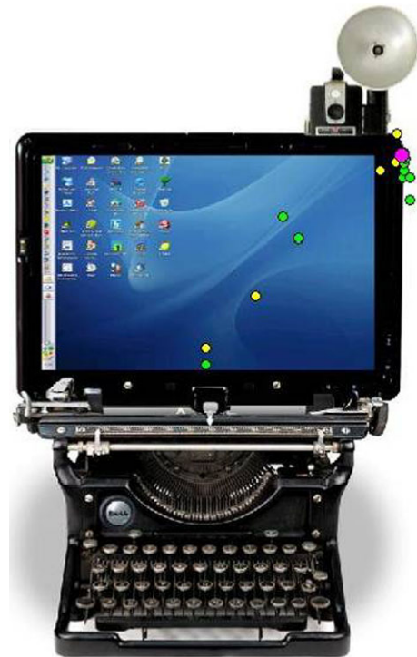
Fig. 14 (Color online) Calculating image center. The yellow dots show convergence of centers calculated before outlier removal. The green dots depict centers after outliers have been removed. Magenta colored dot (at top right corner of the image) depicts the final calculated center. Original image from www.worth1000.com
