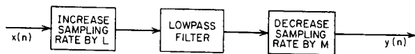
Fig. 2.13 Block diagram representation of sampling rate increase by a factor of L/M .
