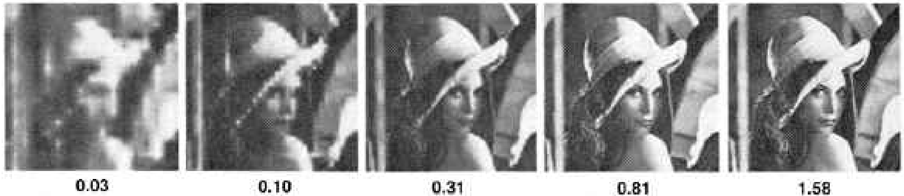
Fig. 9.1. A pyramid code applied to progressive image transmission. High levels of the pyramid are transmitted first to give the receiver a quick but very coarse rendition of the image. The receiver's image is then progressively refined by adding successively lower pyramid levels as these are transmitted. In the example shown here, the leftmost figure shows reconstruction using pyramid levels 4-5, or just 0.03 bits/pixel. The following four figures show the reconstruction after pyramid levels 3, 2, 1, and 0 have been added. The cumulative data rates are shown under each figure in bits per pixel.
