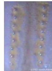
View of the nozzles in a thermal bubble inkjet. (some 300-600 nozzles per head)
