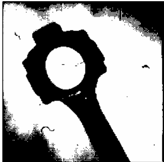
Threshold too high
