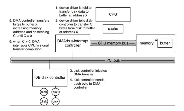
when the DMA controller seizes the memory bus the CPU is prevented from accessing the main memory (but it can still access the caches) — "cycle stealing"
